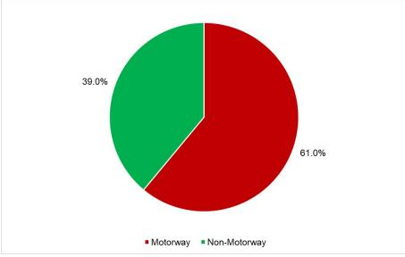
Figure 5: Distribution of Road Types on the TEN-T network
