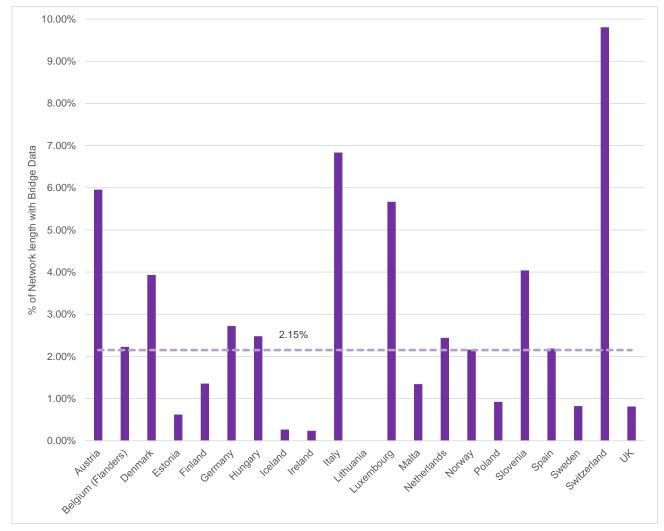
Figure 11: Length of bridges as proportion of total length of national TEN-T network
