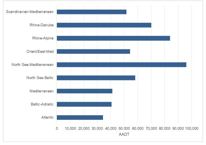
Figure 17: Comparison of Average Daily Traffic Flow on the Core Network Corridors
