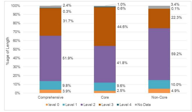
Figure 13: Distribution of ITS on Comprehensive, Core and Non-Core Networks
